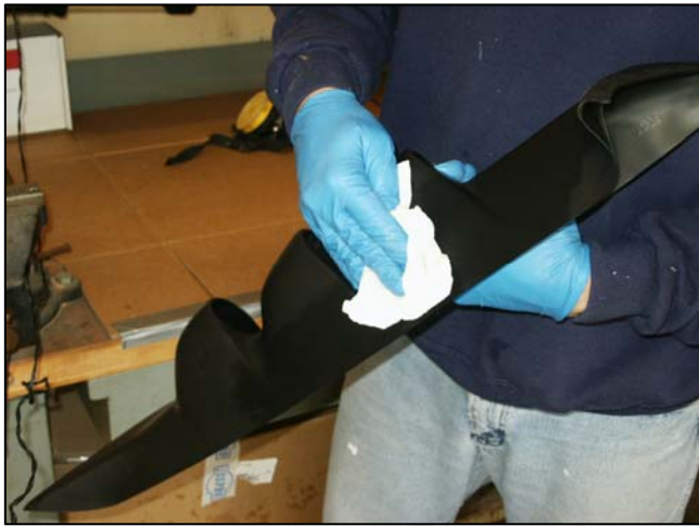
Figure 1) Cleaning with degreaser, wiping in one direction
