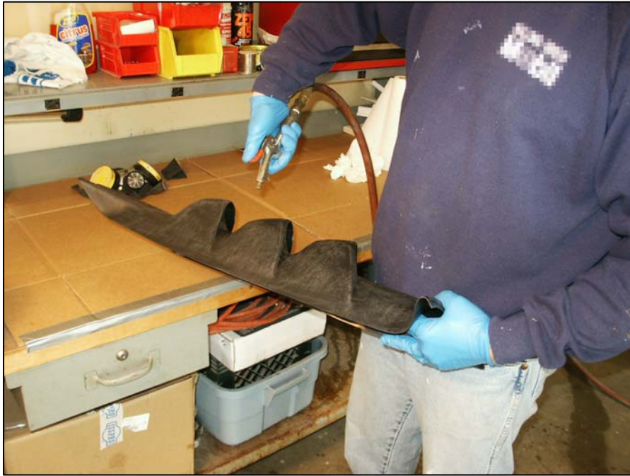
Figure 5) Blow off with compressed air
