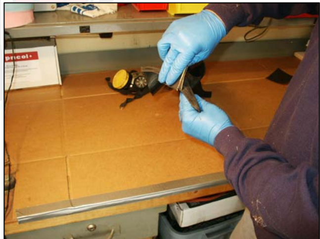
Figure 4) Remove any sharp edges or flashing
