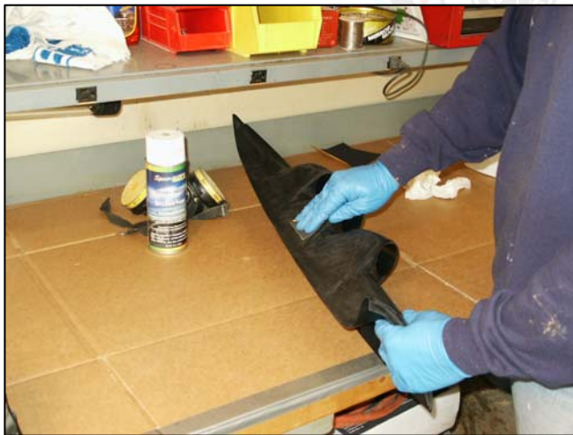
Figure 3) Sand in a small circular motion
