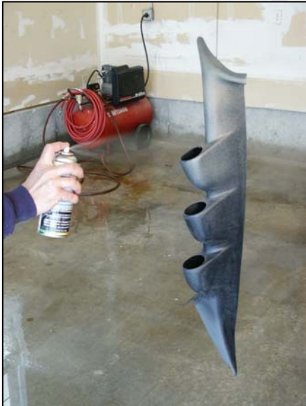
Figure 6) Applying the paint
