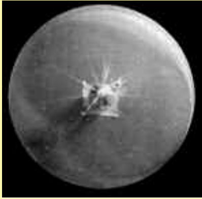
Injector spray pattern without PureFlow®
