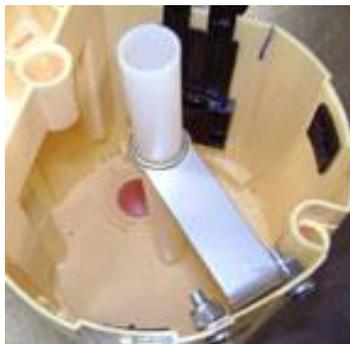
Step 11. Next drill two more holes, one on either side of where the tube will be in bottom of module (fig 11).
