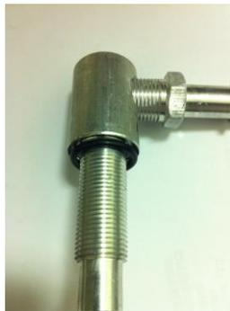
Step 6. Install the washer on the bulkhead fitting first then tighten the Nyloc nut.
