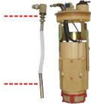
Step4. Remove the unused tube assembly and install the bulkhead fitting using the special grommet adapter.
